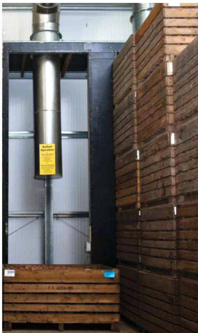
Fig. 3. Open letterbox system used for warming potatoes for the reduction of bruising during washing and grading operations.
